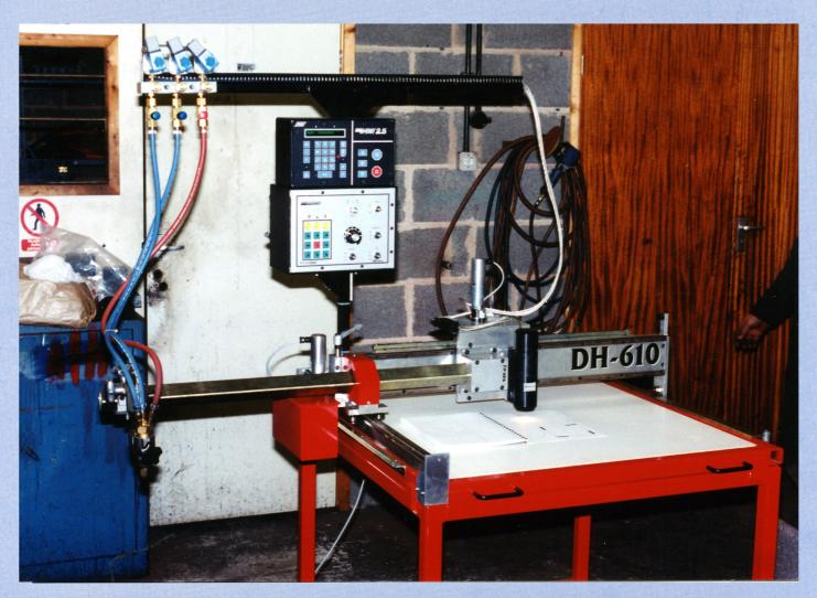
Despite its compact design, the DH610 is a full specification oxy-fuel gas, optically controlled, profiling machine for all general purpose applications.
